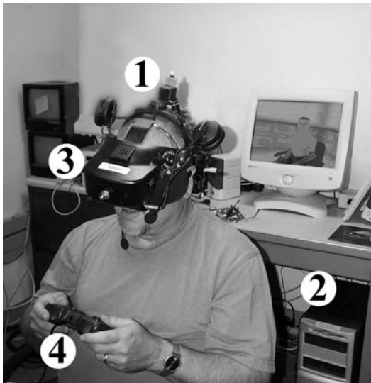
FIGURE 2 A simulated participant wearing the equipment: (1) head orientation tracking device, (2) rendering computer, (3) head-mounted display, (4) game pad used to record responses.
