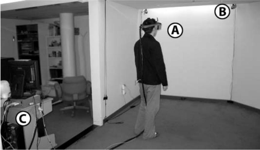
**Figure 1.** Equipment set-up: (A) head-mounted display and orientation tracker, (B) positional tracking camera, (C) rendering machine.
