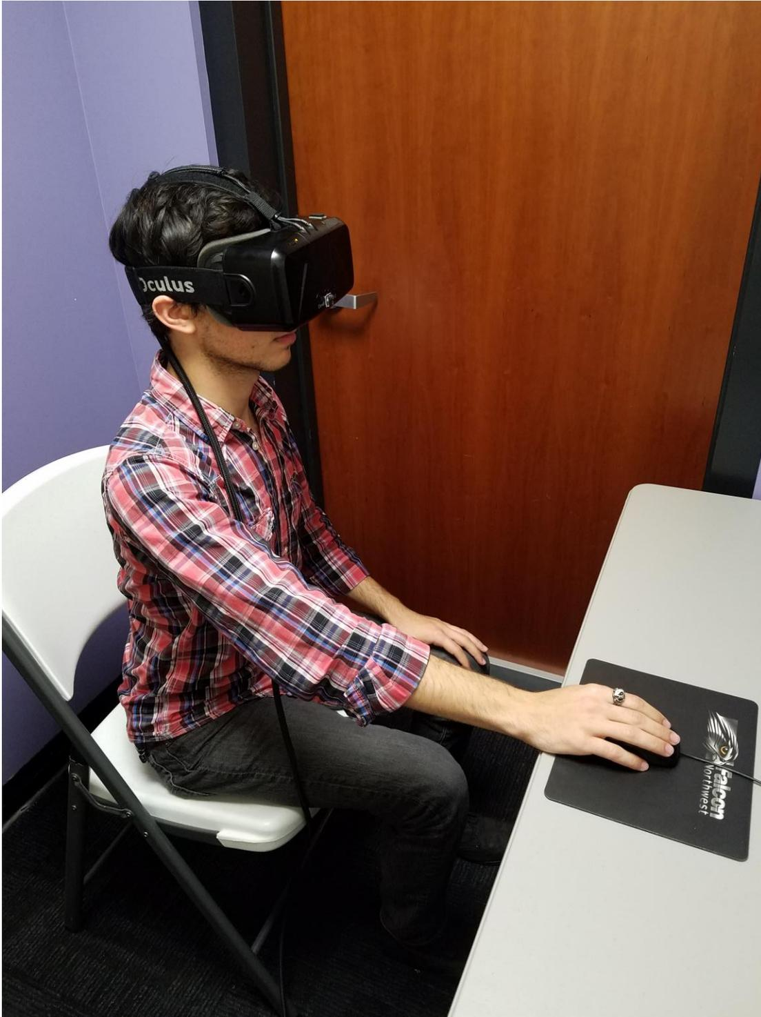
*Figure 1.* A participant wearing an Oculus DK2 VR display, which tracks three degrees of orientation of the user's head with its internal accelerometer and gyroscope.
