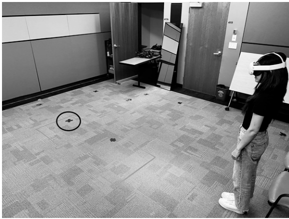
FIG. 2. The participant wears an MR head-mounted display and engages in a blind walk task to the point circled that is 3.12 m away from them. They performed the blind walk task four times (i: in headset, ii: directly after removing headset, iii: without a headset, and iv: without a headset for three more trials after initial no headset).
